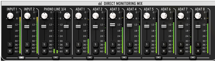
The Direct Monitoring Mix section: 8- channel ADAT view
