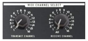
This section allows you to independently set the MIDI input and output channels.
