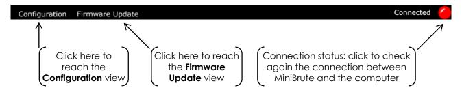
At first launch, the software may detect an older firmware version on your synthesizer, and suggest to update it. It is <u>highly recommended</u> to follow this suggestion, i.e. to run the firmware update process until completion. This is basically the same process as fully described in chapter 3, but it is launched automatically.
