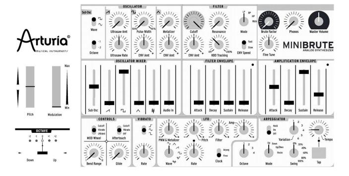
Now set these four envelope sliders all the way down, and raise the **Decay** slider to maximum. Press and hold down a key: the sound appears as soon as you press the key, and slowly fades out to the minimum level. While pressing a key repeatedly, slowly turn down the **Decay** slider: the sound will fade out more rapidly. In the lowest range of the slider, you'll hear short, percussive sounds.
