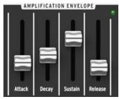
In normal mode, the Amplifier envelope is triggered by the keyboard GATE signal. It can also be triggered by other GATE sources such as the **Arpeggiator** clock [] or the rear panel's external GATE IN jack [4.3.6]. Note that depending on the position of the **GATE** switch located on the rear panel [] the amplifier envelope is under the control of either the keyboard GATE signal, the automatic GATE from the
