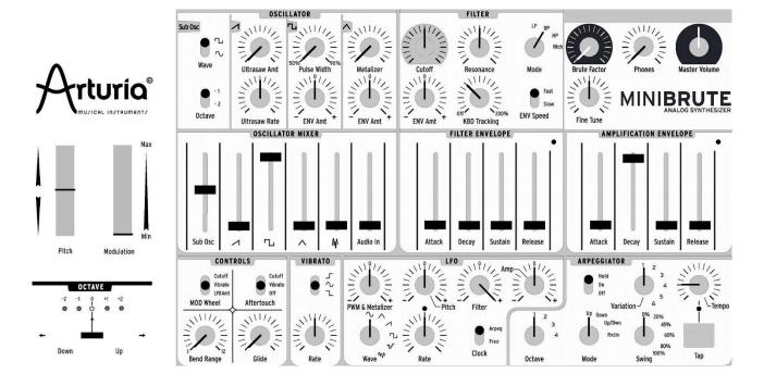
Press the keyboard's lowest C key, then release it: the note auto-repeats continuously, because the arpeggiator is set to **Hold.**
