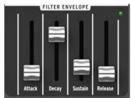
In normal mode, the Filter envelope is triggered by the keyboard GATE signal. It can also be triggered by other GATE sources such as the **Arpeggiator** clock [] or the rear panel's external **GATE IN** jack [4.3.6]. Note that depending on the position of the **GATE Source** switch located on the rear panel [], the filter envelope is under the control of either the keyboard GATE signal, the automatic GATE from the external **Audio input** [4.3.3], or the hold position of the
