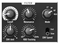
The filter alters the oscillators' timbre via the four response modes described previously (LP, BP, HP & Notch). Its cutoff and resonance can be adjusted manually. The cutoff can also be controlled by the keyboard and modulated by various modulation generators. The MiniBrute filter is based on Nyle Steiner's Sallen & Key architecture (designed in the 70s) and offers - 12dB/octave slopes in LP and HP modes, and -
