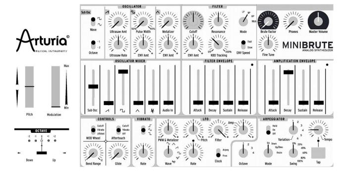
Press and hold a key: you should hear timbre sweeps, a bit like a didgeridoo, at a rhythm indicated by the red LED. Tweak the **Rate** knob to slow down or accelerate this wah-wah effect, and play with the filter's **Resonance** to accentuate it.
