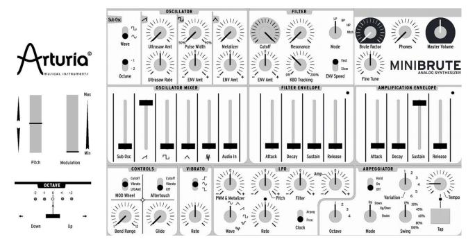
Play the keyboard, and you should hear a basic sawtooth sound rich in harmonics. Next, let's add some animation and life to this flat sawtooth sound. As shown below, turn the **Ultrasaw Amt** fully clockwise. This transforms the sound as if there were two or three slightly detuned oscillators, which creates a slow "beating" effect where the oscillators interact with each other.
