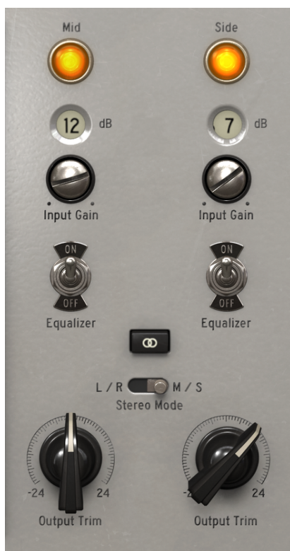
Pre V76 Double Channel Preamp and Output. Notice the Stereo Link and Stereo Mode switches, right above the Output Trim controls, and the Glowing Output Lamps on top
