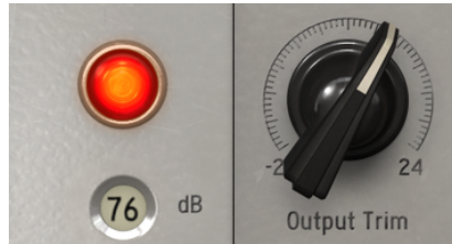
Single Channel Glowing Output Lamp (reaching analog clipping) and Output Trim Knob
