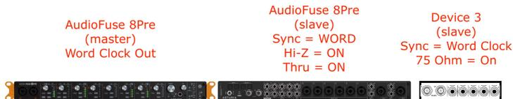
In this scenario there is a third device that can slave to Word Clock. So as with a two-device setup, you don't have to do anything special to the master AudioFuse 8Pre: Simply connect a BNC cable to its WCLOCK OUT connector and run it to the first slave device.
