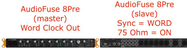
You don't have to do anything special to the AudioFuse 8Pre when it is the master Word Clock device; it is always generating rock-solid Word Clock. Simply connect a BNC cable to its WCLOCK OUT connector and run it to the slave device.
