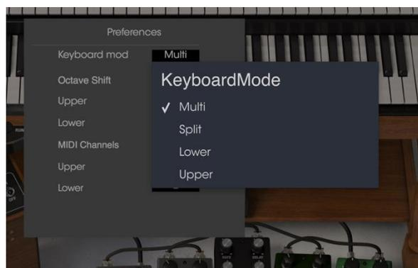
Since B-3 V has two keyboards which generate different tones, we have provided a way to choose how your MIDI keyboard will control the instrument. It provides the flexibility to play both manuals with one keyboard or to use two MIDI keyboards. Here's how it works.
