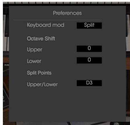
Split mode also allows octave shifting but here you have a single MIDI channel from one MIDI keyboard coming in, and you define which note on that keyboard is the split point at which the MIDI keyboard changes from controlling one manual to controlling the other.
