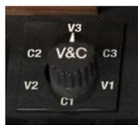
This knob lets you select between three different chorus and three different vibrato types that will be applied to the manuals when their vibrato switches are activated. They essentially represent three different depths for each kind of effect. So C1 is a light chorus and C3 is more intense. Similarly, V1 is light vibrato and V3 is deeper. The three settings could be thought of as Small, Wide and Full.
