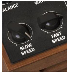
On the speaker module you will find additional controls. The Speed knobs let you set what speeds will be used when the Slow or Fast lever positions (see 3.7.1) are selected. The Slow knob can be set anywhere from 0.100Hz to 2Hz. The Fast knob runs from 2Hz at its minimum setting up to 8Hz.
