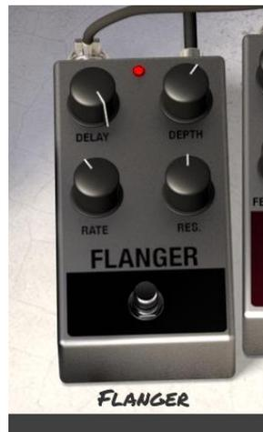
Flanging works by mixing two identical signals together, one signal delayed by a small and gradually changing period. This produces a swept comb filter effect. Here, the controls are:
