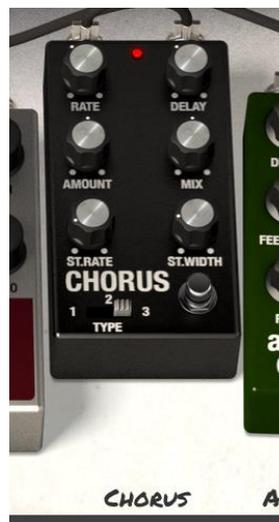
Chorus works by adding a second voice to the signal and in the process making it harmonically richer and adding a sense of movement. The controls are:
