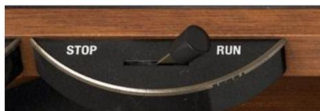
This lever controls whether the rotary speaker is moving or not. In the Stop position, it doesn't add any rotation effect to the sound. In Run mode, it introduces movement based on the position of the Slow / Fast lever and the settings on the speaker itself. If your switch is set to Run while playing, you hear that rotary effect. If you move the lever to the "stop" position, it will act as a brake: the rotary effect will slow down until it stops
