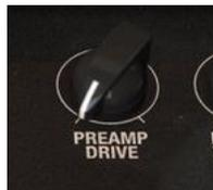
This control can be used to set the amount of drive applied to the preamp. Increasing the amount will add a slightly overdriven effect to the sound, introducing some bite and grit which can be desirable for certain kinds of music.
