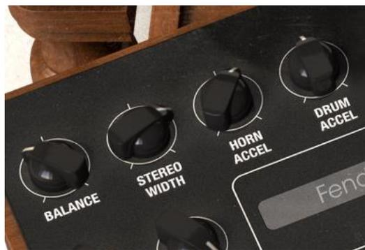
Rotary speakers have two elements: a large drum that deals with lower pitched sounds, and a smaller horn that handles higher tones. The two of these rotate separately which is what gives the sound such unique character. Here there are four controls.
