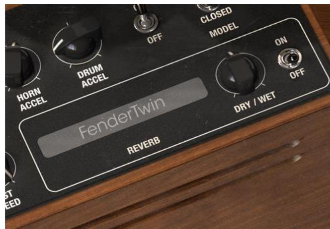
The area contained within the white border is the reverb section. You can switch it on or off, control the dry / wet level and also click on the reverb name to select from one of the other included reverb types.
