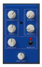
A Compressor reduces the volume of the audio signal above a defined threshold which has the effect of smoothing out volume differences between loud and quiet sections. By making the louder sections quieter, this allows you to apply additional gain to the signal to make the quieter sections louder. The Compressor is a very useful tool for creating a more balanced sound that sits well in a mix.
