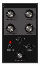
Chorus works by taking an audio signal and mixing it with one or more delayed and pitchmodulated copies of itself, making the sounds harmonically richer and adding a sense of movement and space.
