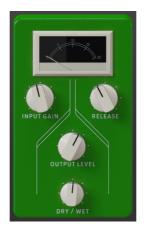
The Limiter is a type of compressor that serves a very specific purpose. It essentially works as a volume "ceiling" to prevent the signal from going above a certain volume. This is especially useful when working with sounds with a wide dynamic range and many effects that could potentially cause the signal to clip and result in clicks and pops.
