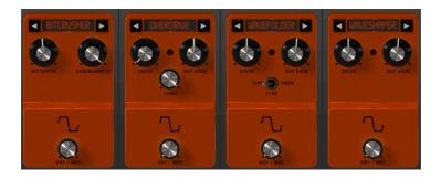
This pedal offers 4 different types of distortion, ranging from subtle drive, crunch and grit to extreme distortion, fuzz and bitcrushing.
