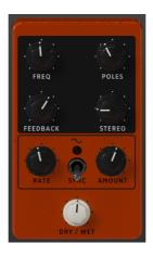
Phasing is the psychedelic sweeping effect that was popular in the 1960s and 70s and adds a sense of movement and swirling to the sound. It works by creating a copy of the input signal, feeding it through a series of all pass filters which create peaks and valleys in the frequency spectrum, then mixing it back with the original signal. As the all pass filters are modulated, frequencies that are out of phase cancel each other, producing the phaser's characteristis "whoosh" sweeping effect.
