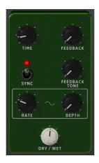
Analog Delay is another type of delay pedal with a slightly different sound. The principle is the same - the input audio is recorded and played back after a small amount of time. A feedback circuit then introduces more copies of the delayed audio back into the original signal.
