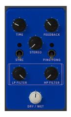
Delay adds dimension and spaciousness to the signal, by creating echoes that can be spread over the stereo image. When using longer delay times, this can also add a rhythmic quality to the sound, especially when working with sounds that have a more pronounced attack.
