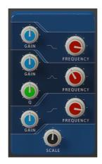
An equalizer is a bank of filters where each filter works in a specific band of the frequency spectrum, boosting or cutting those frequencies to change the overall spectrum balance. It can be used for subtle tone adjustments, or for accentuating certain bands to allow them to cut through the mix.
