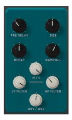
The Reverb pedal allows you to place the sound in a virtual space. This is an algorithmic Reverb, unlike the Room module at the end of the effects chain which is convolution-based. However, this Reverb can be placed anywhere in the signal chain, so that other effects can be applied to the sound after it has been processed by the reverb.
