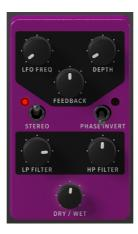
The Flanger works by mixing identical copies of the input signal, with one signal delayed by a small and gradually changing amount of time. While the Chorus works with longer delay times, the Flanger uses much shorter delay times which produces a characteristic undulating swept comb filter effect.
