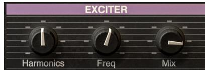
Here is the main attraction of Bus EXCITER-104. It adds harmonics and a substantial high-frequency boost to the signal as described in the [introduction \[p.3\]](#) without adding gain to the throughput signal.
