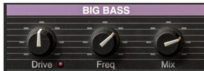
Big Bass replicates the hardware Exciter's "Big Bottom" function, which used parallel compression – meaning it combined a compressed signal with the original – to enhance low frequencies.
