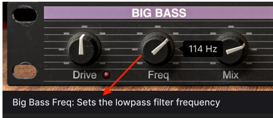
Operating or hovering on any control also displays its name and a brief description of its function in the left corner of the [lower toolbar](#) [p.21].
