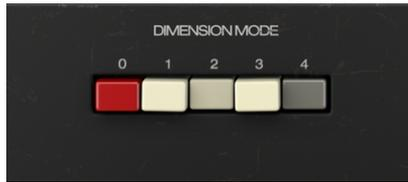
So, to sum it up: you have three chorus intensity buttons, where  $3 > 2 > 1$ , and when you activate the fourth button, you add more wet signal to the mixed output, which means a more chorused signal (more Wet and less Dry signal). Plain and simple.
