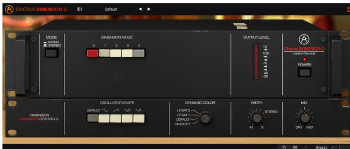
We kept the user interface's simplicity. As is usual with the effect plug-ins produced by Arturia, the Graphical User Interface (GUI) has two panels, the Main panel and the Advanced panel.
