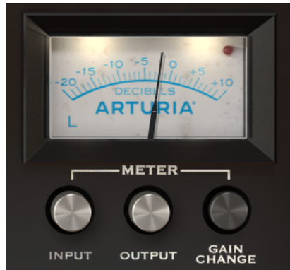
Comp VCA-65 Meter, showing the Gain Change
