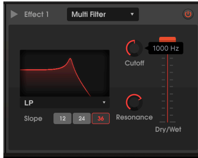
In LP (Low pass filter) mode with a slope of 36 dB/octave and a fairly high resonance
