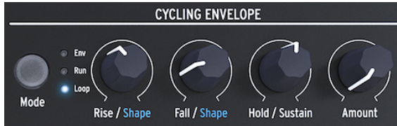
Der Cycling Envelope-Generator
