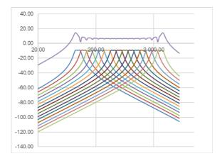
Selecting the frequency range to which the vocoder responds also helps to tune it to male and female voices. Or, when using an instrument as a modulator, to match the vocoder to the frequency range of that instrument.
