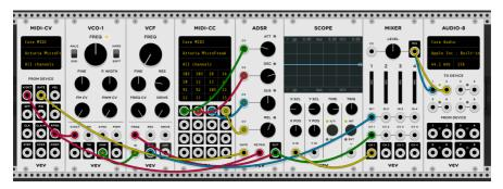
That's it: you have linked the Cyclic Envelope Generator to the VCVRACK ADSR. Whatever changes you make on the Cyclic Envelope Generator will be mirrored on VCVRACK. To hear the effect, press the ARP button the MicroFreak, play a chord and wriggle the knobs of the cyclic envelope.
