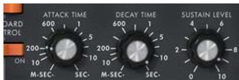
Envelope generator associated to the filter
