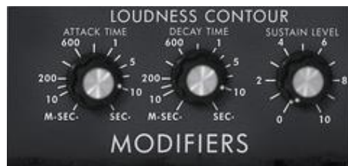
Parameters of the envelope generator associated to the VCA
