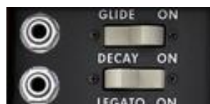
Activating the portamento and return to zero of the envelopes by pedal
