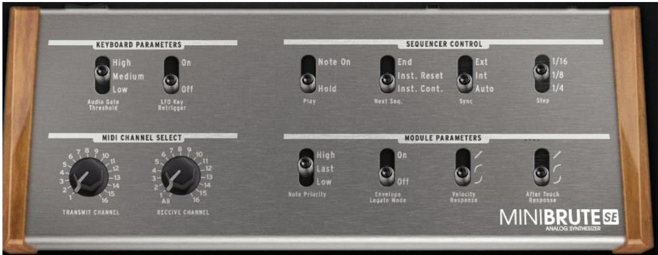
🔑 When changing a parameter, the settings are automatically sent to the synthesizer and stored in its non-volatile memory. No need for saving or reboot, the new settings apply instantaneously!
