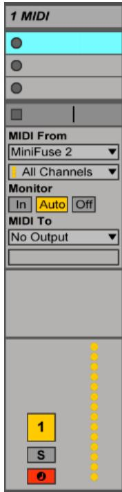
Click the channel's **Record Arm** button. Now when you adjust controls or press pads or keys on your connected MIDI device, you should see the MIDI activity bar light up to indicate that this channel is receiving MIDI. Depending on the software device loaded onto the channel, you should also hear sound being produced from it.
