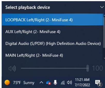
Once you change your system output to use the Loopback output, you will not be able to hear any computer audio until you a) record-enable a channel in your recording application, or b) switch the output back to 'MAIN Left/Right' from the Speaker icon in the taskbar.
