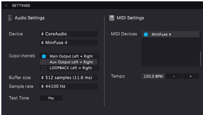
In the **Output Channels** section select Main Output Left + Right; this is the main speaker output from the MiniFuse.
