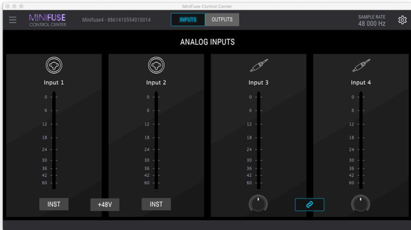
**i** Any settings that you set in the MiniFuse Control Center application are stored in hardware memory and will remain active even after closing the application.
