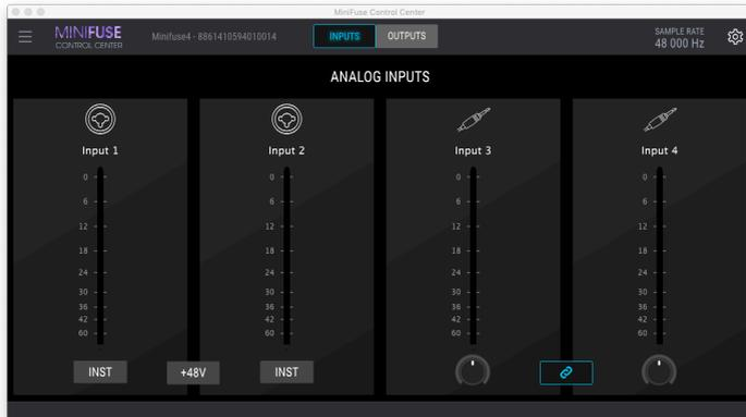
You can either start the application from your computer, or you can press the Arturia switch on the front panel of the interface to bring up the application at any time.
