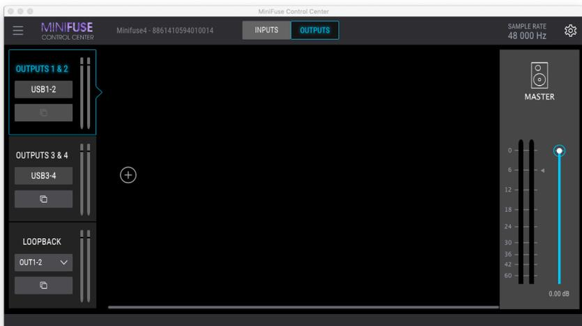
**i** Any settings that you set in the MiniFuse Control Center application are stored in hardware memory and will remain active even after closing the application. On top of that, even if the MiniFuse 4 is not plugged into a computer, the parameters you have set into the MFCC are saved.
