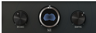
Rev Intensity Distance, Size, and Damping controls. The Size control occupies the center of the Main Control Panel, and has a bigger size. It also displays a graphical representation of the reverb action.
