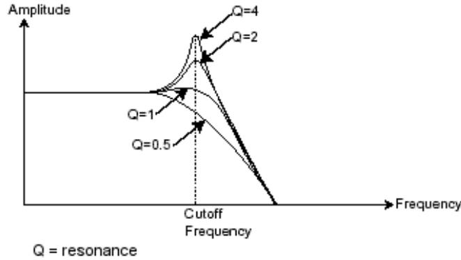
With a very high resonance level, the filter will begin to self-oscillate, creating sound which is close to a sine wave. At this stage, using a key follow on the filter frequency is very important, since it will allow you to play a melody with correct tuning.
