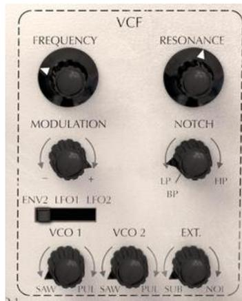
The audio signal generated by an oscillator (the waveform) is then usually directed to a filter module (**Voltage Controlled Filter**). It is this module that we use to control the sound by filtering (by subtraction, which explains the name given to this type of synthesis) the harmonics situated around a cut-off frequency. It can be seen as a sophisticated equalizer that reduces, depending on the case, the high or low frequencies of a sound.
