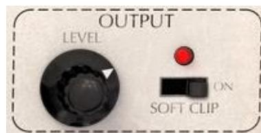
The Level or Master Volume knob adjusts the final output level of the audio signal. It can range from -80dB to +24dB, so be careful, because it may cause audio clipping if set too high.
