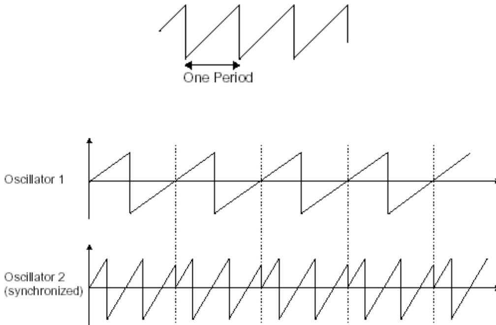
In the above image, oscillator2 is synchronized with the first oscillator and tuned to double the tonality. The resulting waveform is unique in that it cannot be created by standard synthesis techniques such as layering or filtering.
