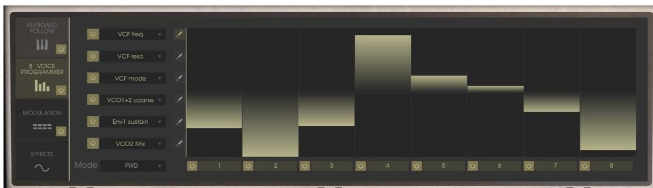
The 8 Voice Programmer module of the SEM V allows you to change the value of up to 6 parameters according to the current state defined by the “board” (see 2.2). The word board references the Circuit Boards used in the original polyphonic SEM-based synthesizers to give it 2, 4 or 8 separate multi-timbral voices. With this module, you can think of the SEM V as an 8-Voice synthesizer, where each voice can play a different sound, opening up an entire world of multi-timbrality.
