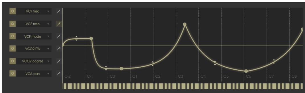
The Keyboard Follow module of the SEM V allows you to modify the value of up to 6 parameters according to the note that is played on the keyboard. It does this by letting you draw the curve of 'reactivity', so to speak, between the pitch of the note and the parameter modulated.
