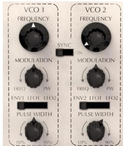
VCO is an oscillator which generates the fundamental audio signal to be processed. There are two VCO sections in the SEM V, named VCO1 and VCO2.
