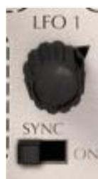
LFO 1 generates a sinewave for modulation purposes. The frequency knob sets how "fast" the LFO is running. If you turn the switch to the "on" position, the frequency will be synchronized with the host sequencer's tempo and you can set the ratio between 1/32 to 16 times the host tempo.
