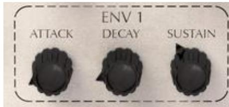
ENV is an abbreviation of Envelope. It creates a modulation shape that is used to control the VCA amplitude, or volume, of each SEM V voice. This shape is generated every time a note is played, and the three knobs present in the ENV1 section (Attack, Decay and Sustain) help determine the shape of the envelope.
