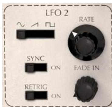
On this LFO, you can choose the modulation waveform by using the upper switch: either sine, sawtooth or square.
