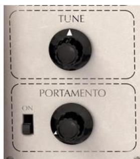
TUNE controls the master tuning of SEM V within A=420Hz to 460Hz.
