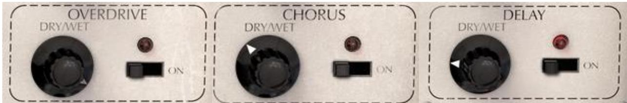
SEM V has 3 kinds of effects (Distortion, Chorus and Delay). You can turn them on or off by using the switches on the right side and control the dry/wet balance by adjusting the knobs to the left.
