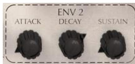
ENV 2 is not directly sent to a SEM V parameter like ENV 1 (sent to the VCA). It can be viewed as an external Modulation source, and can be sent to the filter frequency in the VCF or else to the frequency or pulse width modulation of VCO2.
