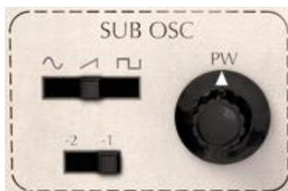
The upper switch determines the wave form of the Sub Oscillator, either sine, sawtooth or pulse. You can choose the pitch to be either of 1 or 2 octaves lower than VCO 1's pitch. The knob on the right side controls the width of pulse wave.
