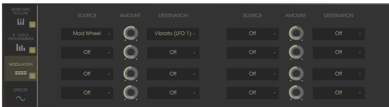
Thanks to this feature, you can modulate many parameter values by several control sources such as Pitch bend, Modulation wheel, Velocity, Aftertouch, LFOs and Envelopes.
