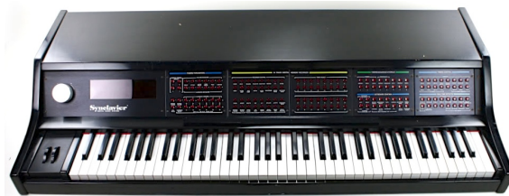
Velocity/Pressure Sensitive Keyboard (VPK)
